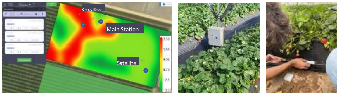
Figure 2: Definition of the location of the monitoring points in the PILOT plot (a), communication node installed in the plot (b) and installation of sensors in the different monitoring points (c).
